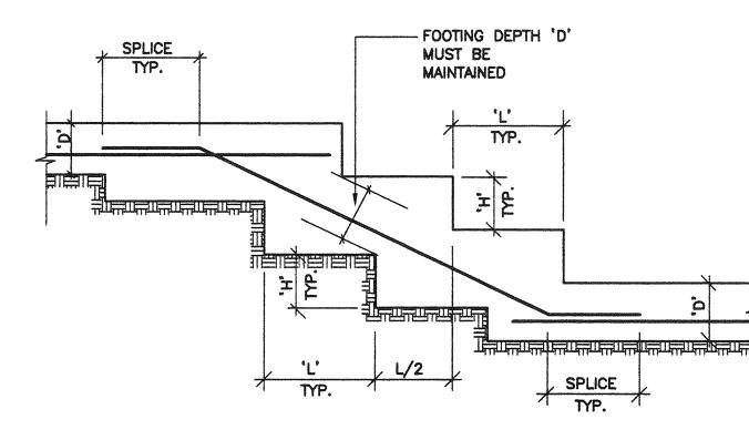
H = 1'-6" MAX.L = 2H MIN.D = DEPTH OF FOOTING SEE PLANS & DETAILS
